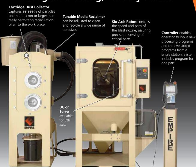
Empire's new RBT36-F robotic pressure-blast system opens the door for many firms to cash in on the benefits of high precision air blasting. Capable of processing parts up to 12 inches in diameter by 12 inches tall, the RBT36-F employs a Fanuc 6-axis robot to control nozzle movement plus a DC or Servo drive to control part movement, enabling users to assure the quality control and deliver the process validation so often required by today's aerospace, automotive and medical-equipment sectors.
